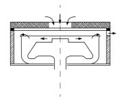
Limited ventilation on the upper side of the rotor
