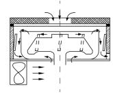
Double cooling air design, enforcing air cooling from both the upper and lower side for the rotor.
