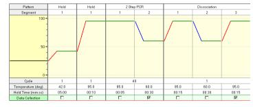
Stage 1: Reverse Transcription Hold 42°C 5 min 95°C 10 sec Stage 2: PCR reaction Repeats: 40 times 95℃ 5 sec 60°C 30 sec Stage 3: Dissociation
